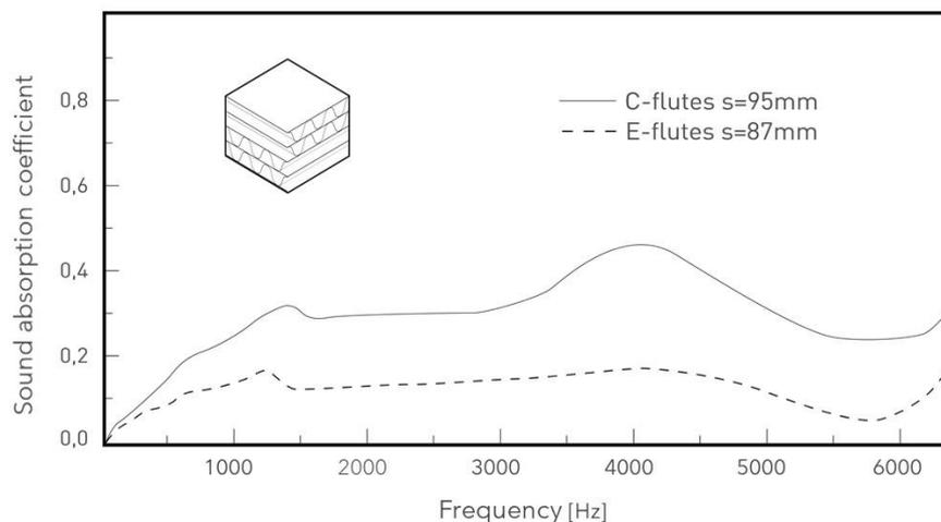
Fig. 1 Sound absorption coefficient of the multi-layered corrugated cardboard, with wave incident on a cover [5]
