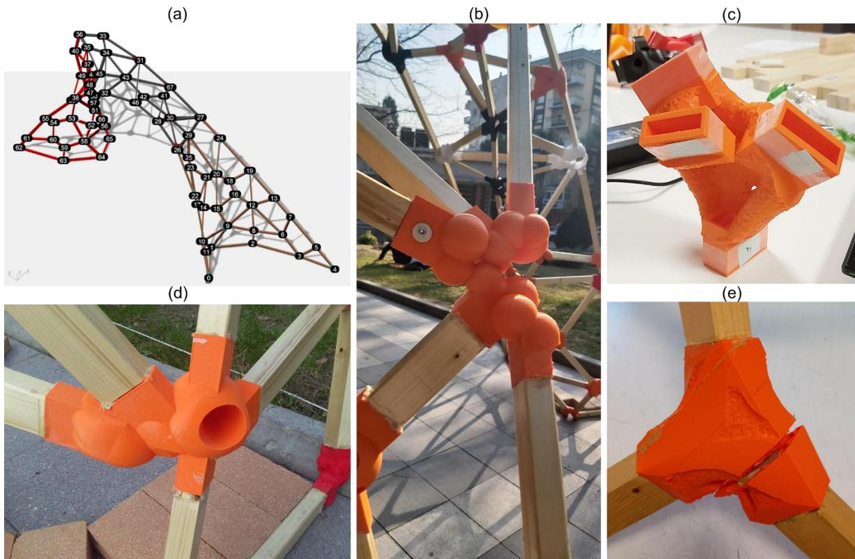
Fig. 2. (a) Digital model of *the Gate*; (b) example of a 5-bar node design; (c) the connecting boxes; (d) example of a potato with a hole; and, (e) a broken node.
