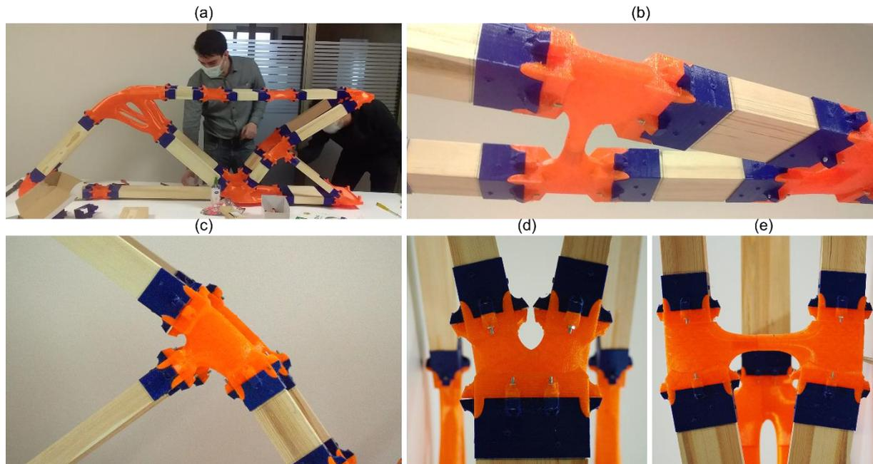
Fig. 3. (a) Full scale model of the cantilever; (b) example of a 4-bar two-piece node; (c) a node connecting bars; (d) a 4-4-6 node; and, (e) a 4-4-4-4 node.
