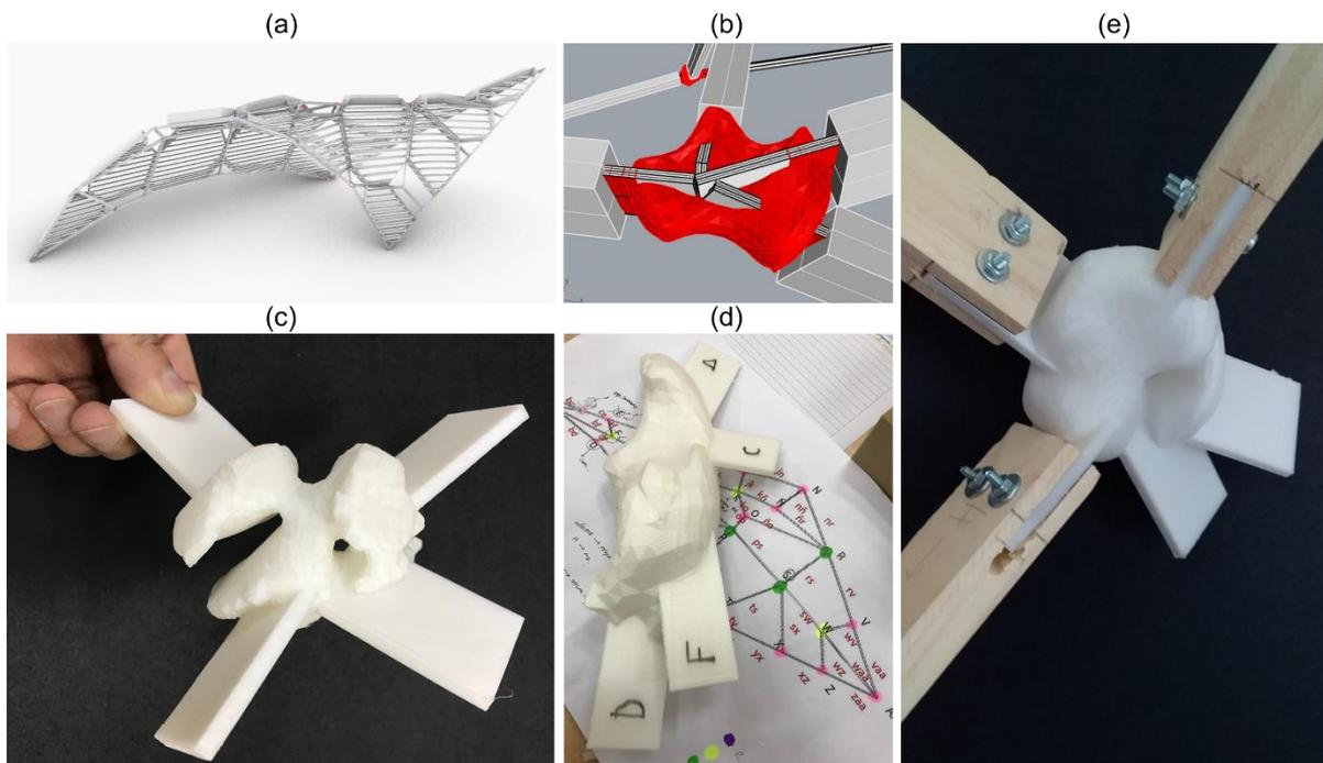
Fig. 1. (a) Digital model of the shading artifact; (b) example of a 4-bar node design; (c) a topology optimized node; (d) the first potato; and, (e) a node with timber battens.
