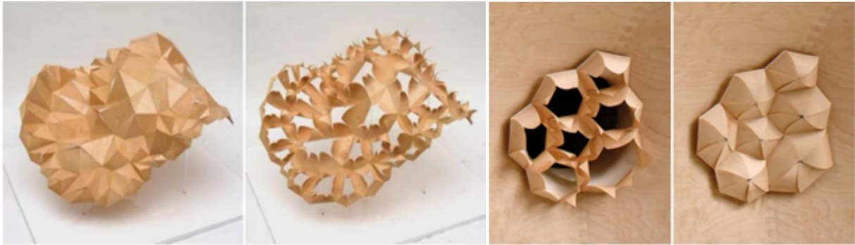
Fig. 1. Responsive wood-composite structures reacting to changes in ambient relative humidity
