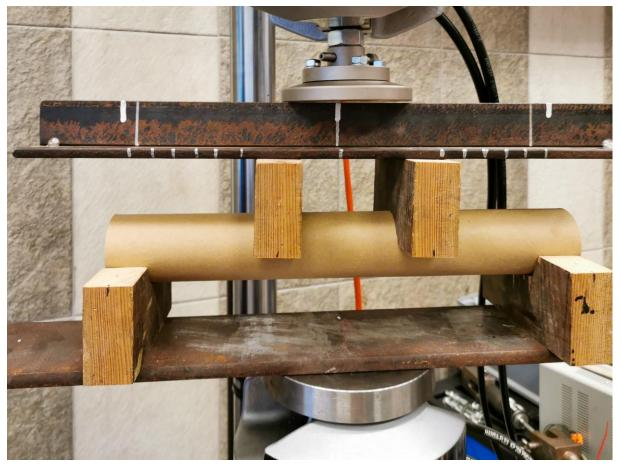
Fig. 1. Structural tests on paper tube
