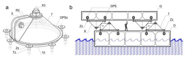
Fig. 2. a) View of the conical body equipped with a rack and pinion stabilizing ring (OPSz), b) vertical section of a floating platform designed as a power station.
