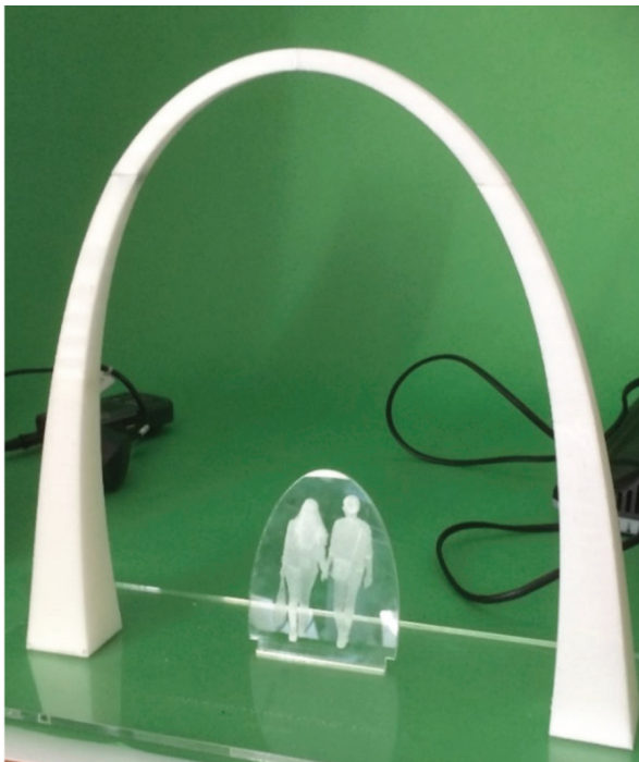
Fig. 3. Constant stress, free-standing arches. Input: span and rise: 6 m, cross section area at the apex: 0.3 \text{ m}^2 , concrete of mass density 25 \text{ kN/m}^3 . Output: arch profile, varying cross-section area, constant stress: 0.049 \text{ MPa} .
